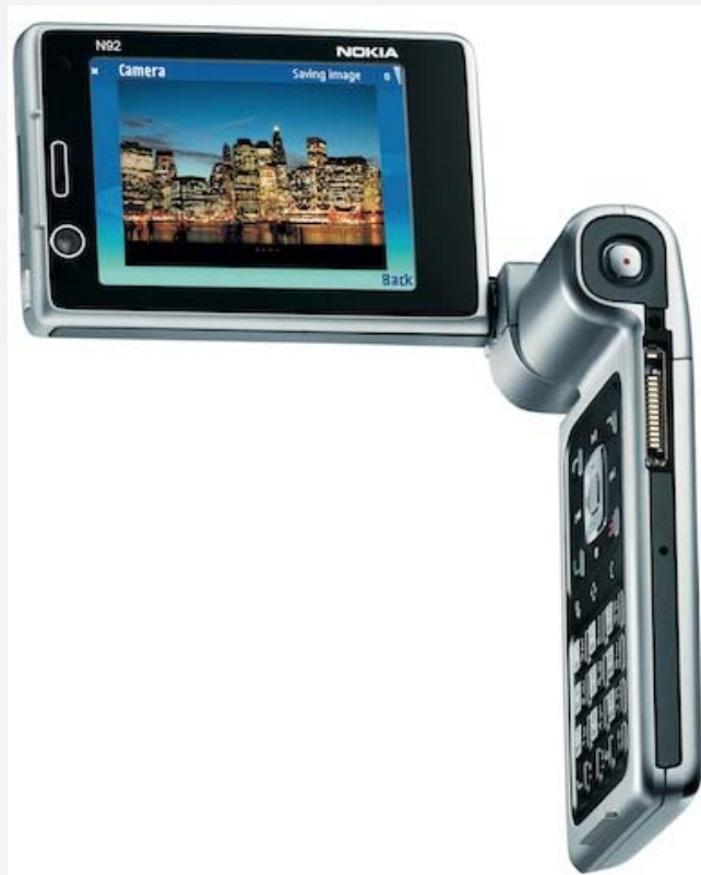
Figure 4: Advanced mobile devices have axis movements that add mechanical stress to interconnects between the display and processor (Source: Nokia Corporation)
