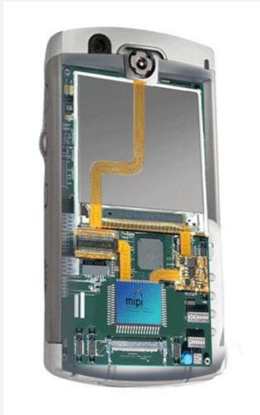
Figure 1: Inside of a mobile phone showing an example of MIPI connections between the application processor and camera and display subsystems.
